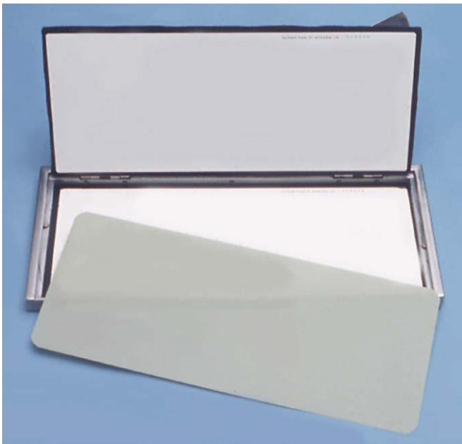
FIGURE 5-9 Cassette for 8 inch \times 10 inch film along with a sheet of screen film. When the cassette is closed, the film is supported in close contact between the two white intensifying screens seen on the inside of the cassette. These intensifying screens absorb most of the incident x-ray beam and then fluoresce and expose the film.
