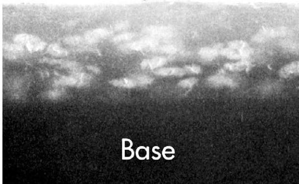
FIGURE 5-17 Scanning electron micrograph of a processed emulsion of Ultra-speed dental x-ray film (500 \times ). Note the white-appearing solid silver grains above the base. (Courtesy of Carestream Dental, a division of Carestream Health, Inc.)
