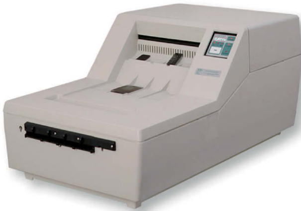
FIGURE 5-23 Dent-X 810 AR film automatic film processor. The operator opens the film packet in a darkroom and inserts the film into the opening on the left end of the machine. The exposed film is carried on a roller apparatus through processing solutions, and the processed and dried film is returned through the upper right opening in 4.5 minutes. (Courtesy ImageWorks, Elmsford, NY.)
