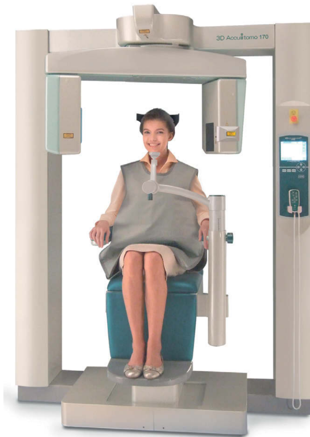
FIGURE 11-1 Example of CBCT unit. Imaging may be performed with the patient seated, supine, or standing. The patient's head is positioned and stabilized between the x-ray generator and detector by a head-holding apparatus. The detector may be a flat panel (this example) or image intensifier. During exposure, the generator and detector rotate fully or partially around the patient's head. Scan time may be as fast as 5 seconds. A separate exposure parameter control panel may be displayed either on the computer screen or on the equipment itself (as shown). Most CBCT units have a small "footprint" enabling in-office placement. (Image of 3D Accuitomo 170 shown courtesy of J. Morita Mfg Corp, Kyoto, Japan.)
