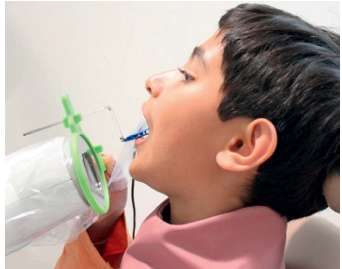
FIGURE 3-8 Rectangular collimation. Another means to collimate a round beam to a rectangle is to place a metallic shield in the path of the beam, limiting the size of the exposure field to an area just larger than the film or sensor. The JADRAD Dental X-Ray Shield is shown. (Courtesy Dr. Jennifer Diederich, Farmington, CT.)
