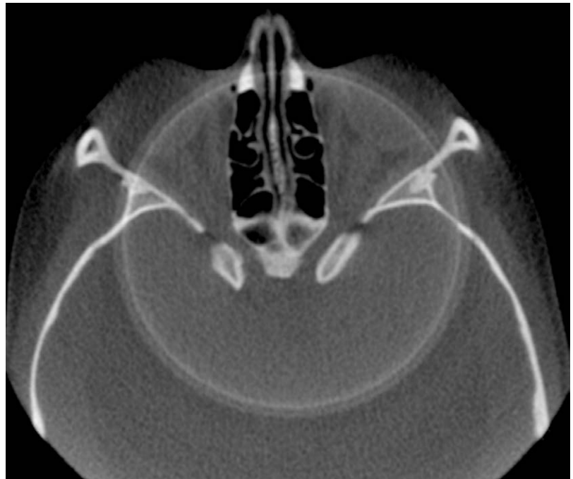
FIGURE 11-14 Circular or ring artifacts. Visual appearance of scanner-related artifacts as circular rings on an axial image suggests imperfections in scanner detection as a result of poor calibration.
