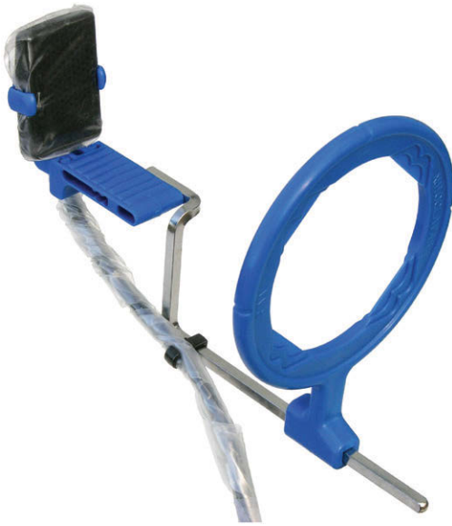
FIGURE 3-6 XCP film-holding instrument. The aiming ring aligns a circular aiming cylinder from an x-ray machine with the sensor to ensure that the image plane is perpendicular to the central ray and in the middle of the beam. Note notches to align rectangularly collimated aiming devices, such as shown in Figures 3-5 or 3-7. The digital sensor and cord is in a plastic bag to prevent contamination from saliva. (Courtesy Dentsply Rinn: http://rinncorp.com .)
