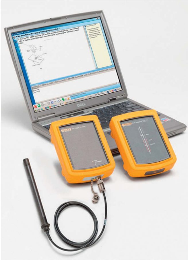
FIGURE 15-4 Device for measuring exposure output of an x-ray machine. The probe on the left is intended to be included in a phantom to measure cone-beam computed tomographic exposure. The aiming cylinder of an intraoral dental x-ray machine may be positioned over the center of the device on the right, and an exposure may be made. These units measure average and maximum kVp, dose, dose rate, HVL, and exposure time in seconds or pulses. (Image courtesy Fluke Biomedical: www.flukebiomedical.com .)
